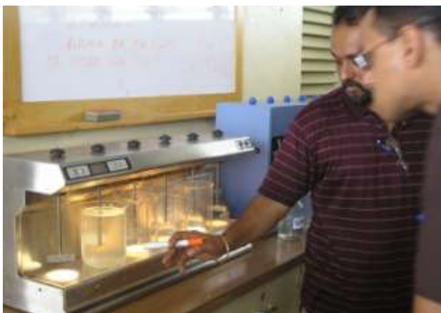
Jar Testing for Correct Chemical Dosing
